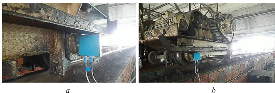
Fig. 4. Placement of acceleration sensors on the axle of the bogie wheels: a – driven wheel; b – drive wheel
