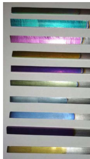
Fig. 3. The surface of specimens made of the Ti6Al4V alloy after their oxidation in galvanostatic mode
