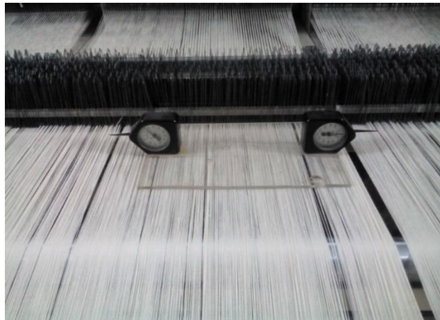
Fig. 3. Instruments for measuring the tension of the main individual yarns on looms
