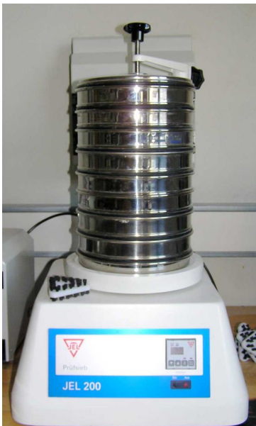
Fig. 1. A series of sieves with different hole sizes and weighing weights of structurally inhomogeneous materials
