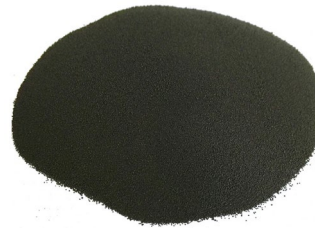
Fig. 2. Full-scale powder bulk materials for forming structurally inhomogeneous materials (aluminum, d = 0,15-0,2 mm, P = 25\% )
