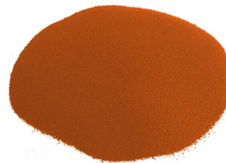
Fig. 3. Full-scale powder bulk materials for forming structurally inhomogeneous materials (copper, d = 0,45-0,63 mm, P = 20\% )
