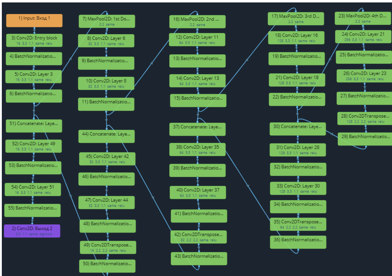
Fig. 2. The architecture of the proposed CNN (basic U-Net) in the Terra AI framework
