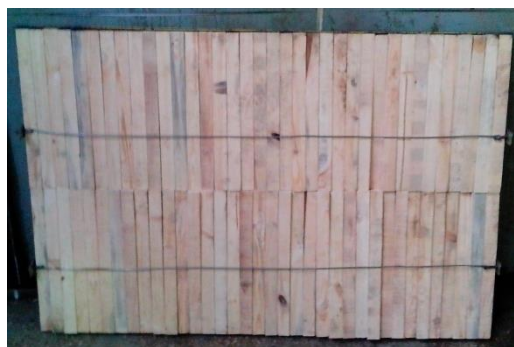
Fig. 6. Imitation of the car floor, which in its fire load is close to the model hearth 1A.
