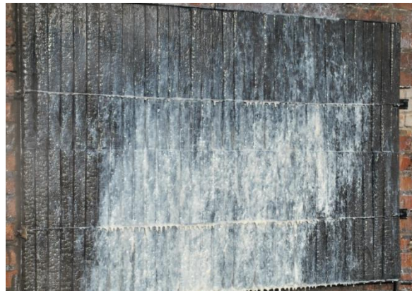
Fig. 8 Adhesion of the gel layer on the surface of the model hearth made of wood
