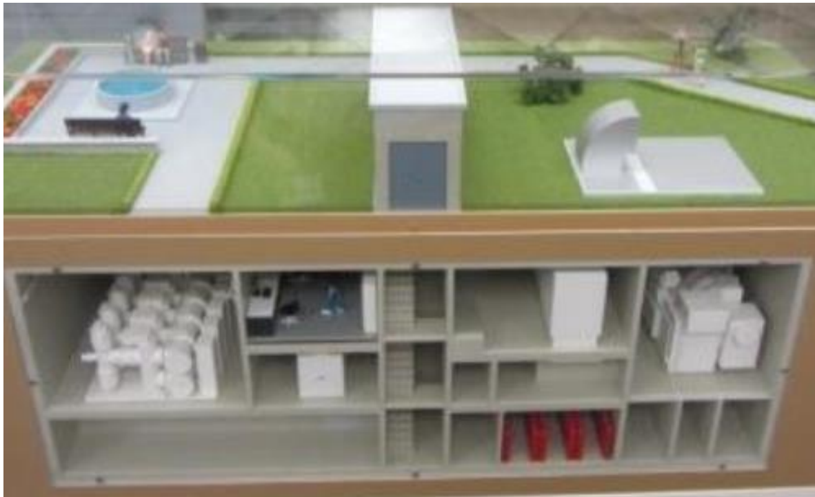
Figure 3. Example of underground SS.
