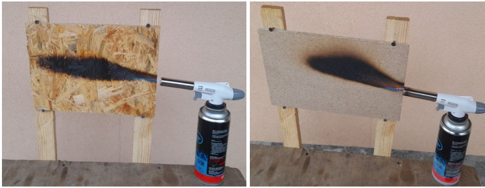
Fig. 3. General pattern of experimental conditions: on the left side we can see the gas burner and the OSB specimen and on the right side we can see the gas burner and the WPB specimen
