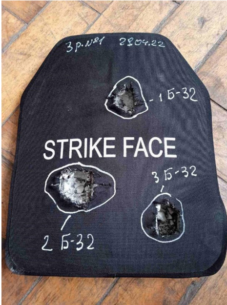
Fig. 4.9. The appearance of a ceramic plate when it is affected by a striking factor
