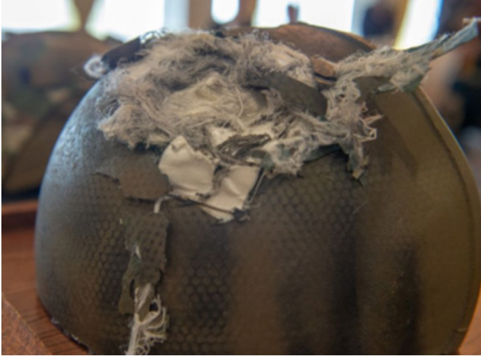
Fig. 4.12. The appearance of the helmet after being hit by fragments 3 cm in diameter
