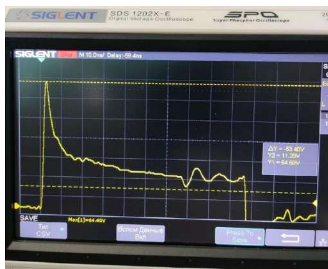
Fig. 2. Volt-second characteristics of the switching process in a cadmium telluride film.
