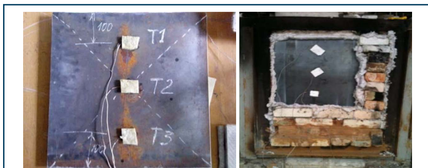
○ Fig. 4.6 Layout of thermocouples from the unheated surface of the steel plate before the test
