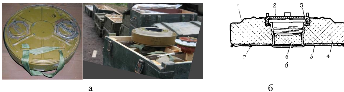
Figure 1. – TM-62M anti-tank anti-tracked high explosive mine of 9.5-10 kg: a – general view of the mine without a fuze (defused); b – section of the mine: 1 – metal body; 2 – plastic plug; 3 – gasket; 4 – explosive (TNT = 7 kg or TGA (MS) = 7.5 kg); 5 – bottom; 6 – pressed grenade detonator (TNT = 0.2 kg); 7 – eyelet for attaching the handle; diameter – 32 cm.; height – 12.8 cm.; (MS – marine mixture). 4 mines without fuzes are placed in a wooden box painted green
