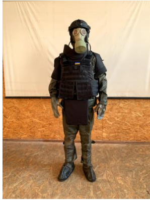
Photo 1. – Combination of L-1 protective suit, armor protection of the IV level of protection type protective body armor, III-A level of protection armor helmet and GP-5 type filter gas mask
