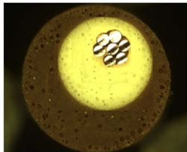
Fig. 12. Concentricity of coating on wire ( h_2 = 0.051 \text{ mm} , wV = 4 \text{ m s}^{-1} , p_t = 150^\circ\text{C} )
