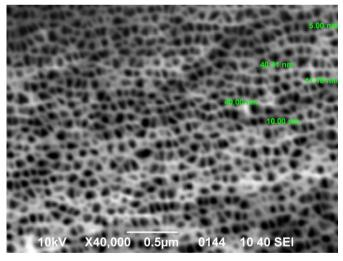
Fig. 5. SEM image of por-InP (surface)
