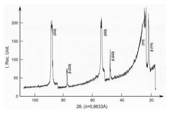
Fig. 7. X-ray spectra porous InP (100)
