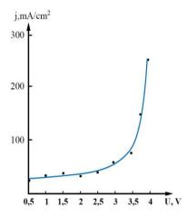
Fig. 3. Dependence of density of a current on a pressure during anodization
