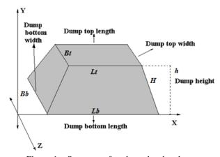
Figure 1 – Structure of coal overburden dump
