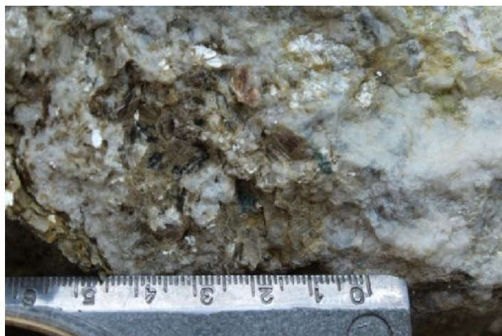
Fig. 8. Pegmatite (albite zone) of Balka Kruta deposit. Pegmatites of Kruta Balka are a small deposit of lithium and tantalum.
